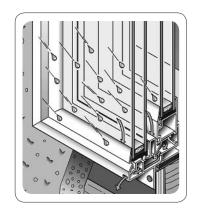
Remove the screen during this cleaning process so that the screen track area in the sill is cleaned and scaled. Clean out your window and door "weep holes" using a small, soft bottlebrush. These weep holes are visible on the inside track areas (both the vent track and screen track) as well as the exterior sill surface of the frame. Be careful not to damage exterior weep hole covers or baffles. Weep holes must remain clean and clear to properly drain water to the outside.
